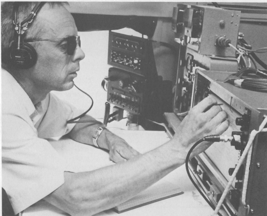
Senior scientist with NOAA's Atmospheric Physics and Chemistry Lab at Boulder, Colorado, points to strip-chart recorder, one of many HP instruments, used in airborne monitoring of surface temperatures, high-altitude water vapor, and clear-air turbulence. This particular aircraft, a NOAA Convair 990, crashed in a golf course less than a mile from HP's Mountain View complex last year. A new 990 with a full complement of new HP gear was recently placed in service.
